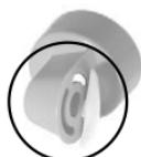
Snap membrane onto valve until membrane lies completely flat.
