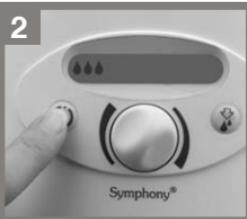
Switch on the breastpump by pressing the On/Off button. The pump will begin pumping in the **Stimulation Phase**.
