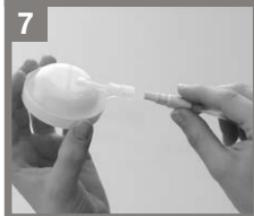
Push adapter end of tubing into opening on membrane cap.
